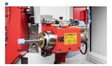
The swiveling wheelhead is equipped with water-cooled, roller-based, and maintenance-free motor spindles with stepless speed control and the latest generation of contact sensors. The shaft ends hold external wheelheads with a diameter of 500 mm (20") and a width of 63 (80 F5) mm (2.48" (3.15" F5)). For internal grinding, use powerful high-frequency spindles with 120 mm (4.72") external diameter. It's your choice: configure the wheelhead to match your specific needs.
