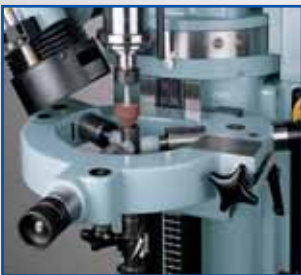
Concentric grinding with the steady rest
