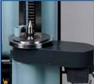
Workpiece drive with two speeds 25 \text{ min}^{-1} / 50 \text{ min}^{-1}
