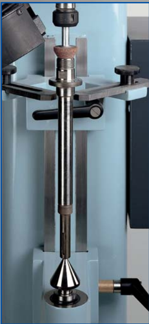
Plunge grinding: The centre hole is laped in full contact.
