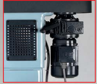
Stepless variable grinding spindle speed for centres upto 120 mm dia
