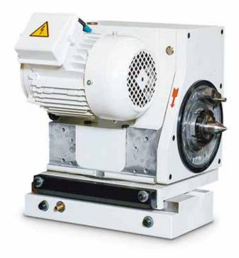
The swivelling workhead with hydrodynamic bearing makes it possible to grind between fixed centres as well as with rotating centres. The powerful workhead spindle, relieved from belt tension, rotates in a hydrodynamic multisurface plain bearing. Roundness during live spindle grinding is 0.0003 mm (0.000,012"), with the option of 0.0001 mm (0.000,004") available. The workhead is driven by a stepped AC motor.
