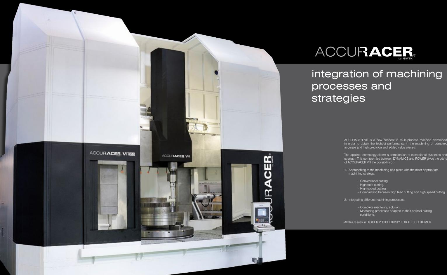
ACCURACER VR is a new concept in multi-process machine developed in order to obtain the highest performance in the machining of complex, accurate and high precision and added value pieces.
